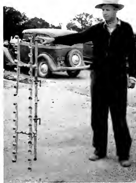
Evans spraybar used in eliminating roadside vegetation alongside State highways
